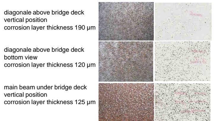
Figure 4 – The different structure of patina layer on bridge after 30 years of exposure
