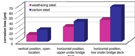
Figure 2 - The corrosion loss of weathering and carbon steels after 12 years of exposure in different positions on bridge structures
