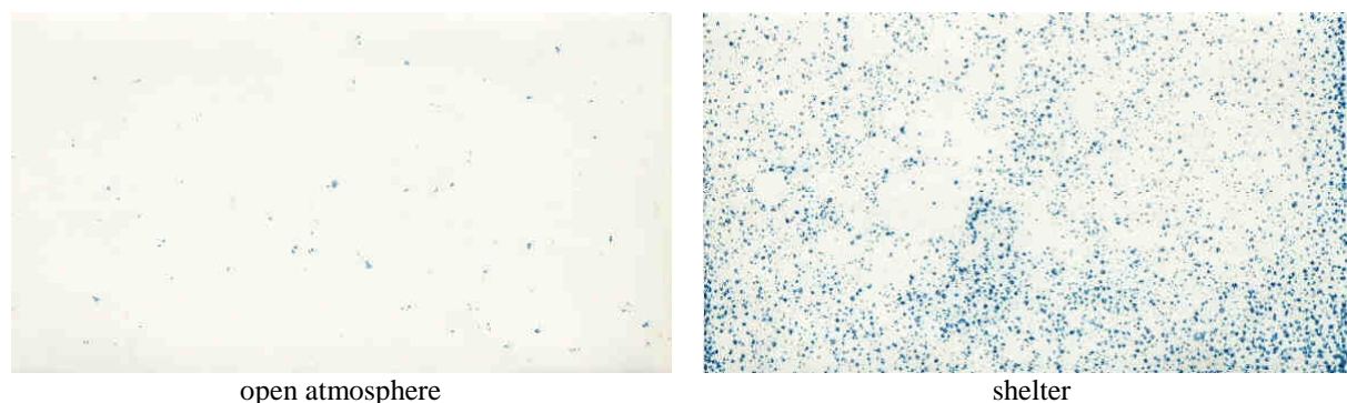
Figure 2: Distribution of sulphates and chloride nests in rust layer after 8 years of exposure
