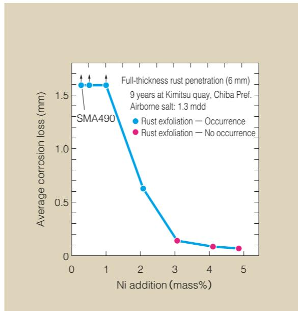
Fig. 4. Secular changes in coastal exposure test (Exposure test at Kimitsu quay, Airborne salt 1.3 mdd)
