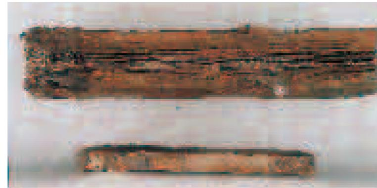
Cross-sections of conventional weathering steel (above) and coastal weathering steel (below), both having a thickness of 6 mm and exposed for 9 years at Kimitsu quay
