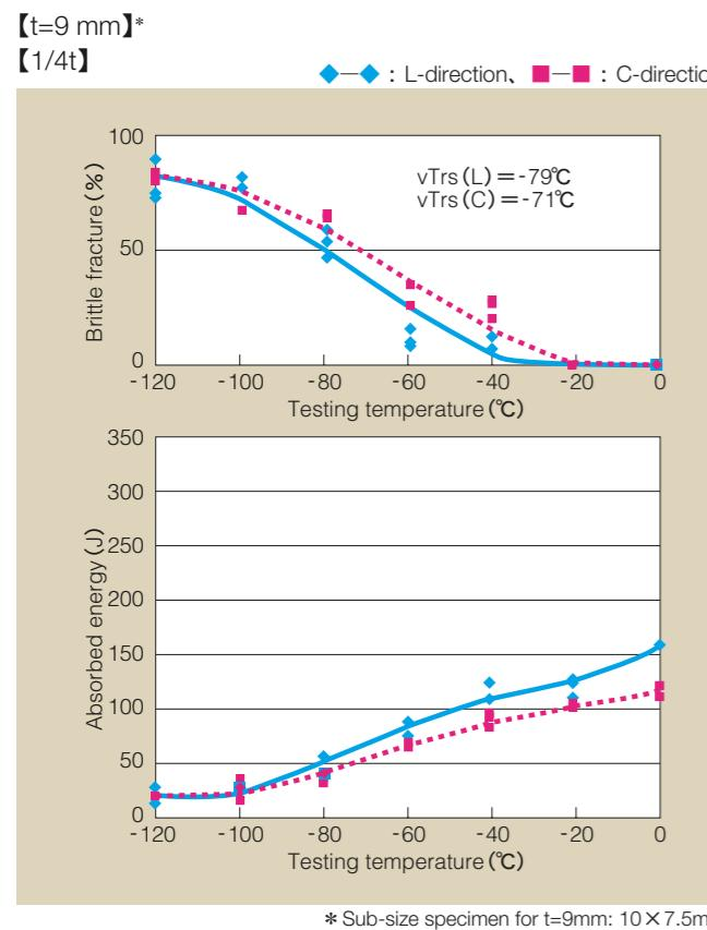
● 570 N/mm<sup>2</sup> grade coastal weathering steel SMA570WQ-MOD
